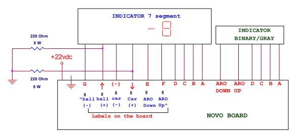
Note: In case of use Arrow up & Arrow Down in 7-Segment only, install 2 resistances (220 Ohm, 5 W) each as shown in the diagram above. (7-segment is active low only)
